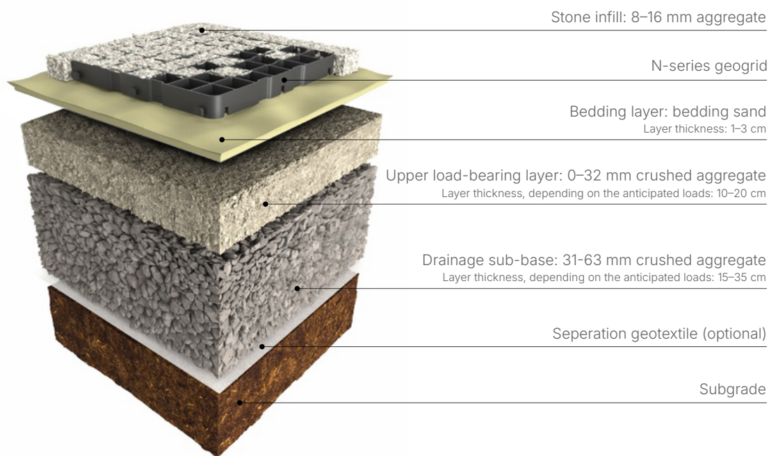
Figure 4 Suggested sub-base build-up
